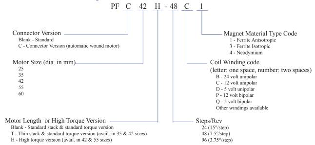
For the gear head motors, the gear ratio is designated after the magnet material type code.
